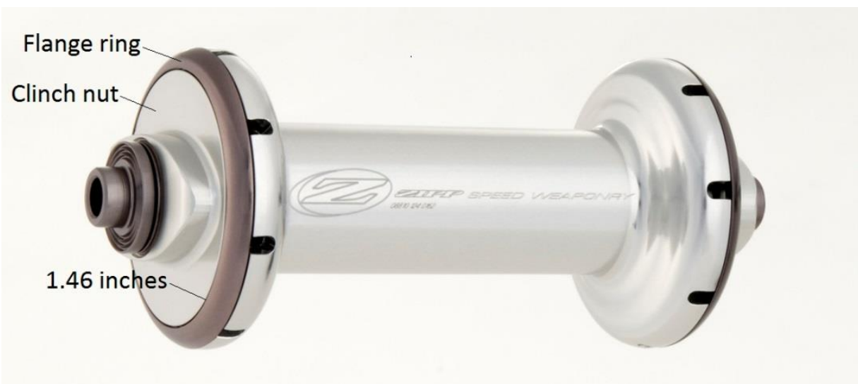
Photo 1: Silver ZIPP 88v6, 88v7 and 88v8 front hub – affected version
